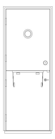
DESCRIPTION: Type 3, Aluminum, Dutch Type, in Halves with Shelf, Alternate Sill
